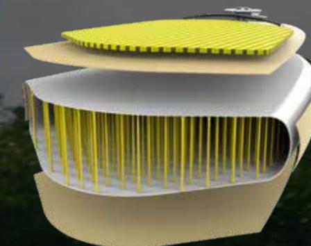
To provide unmatched strength and durability, drop stitch material is a network of thousands of polyester threads. They securely connect the material surfaces internally, which seal in air to keep the board inflated and rigid, yet still lightweight. Drop stitch material can support considerable weight when inflated while still being easily portable when deflated.
